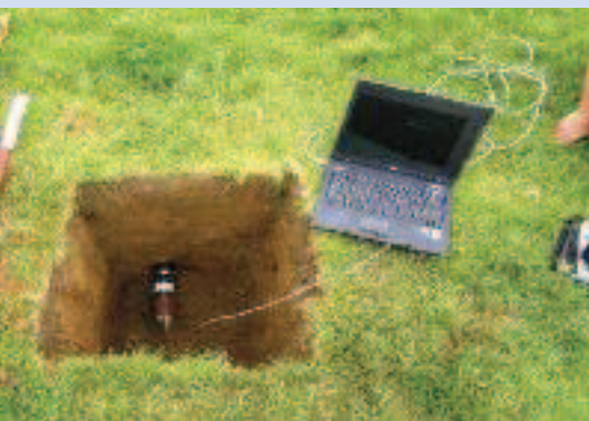
Background radiation being measured by a spectrometer, New Close, Malham, North Yorkshire (SD 911 645)
